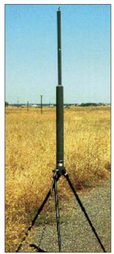
Fig. 1 Tripod-mounted CM201B antenna.
