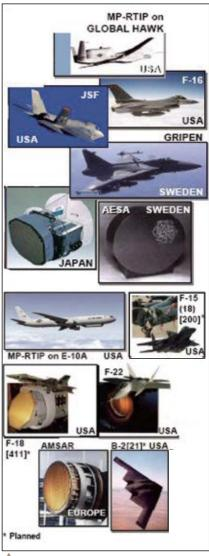
▲ Fig. 6 Examples of airborne MMIC active arrays deployed and under development.
