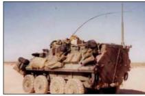
Fig. 4 COM237 antenna mounted on a military vehicle.
