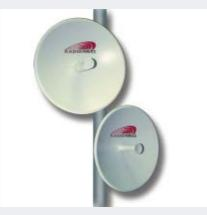
The SPX-3.5NS series of antennas covers a frequency range of 3.3 to 3.6 GHz or 3.5 to 3.8 GHz. Providing coverage down to 3.3 GHz makes these reliable parabolic dishes usable in numerous international bands including China. The standard SPX-3.5NS antennas now cover 3.3 to 3.6 GHz and can be ordered "tuned" to the 3.5 to 3.8 GHz bands when required. These antennas are available in diameters from 2 to 8 feet and accompany a three-year warranty.
